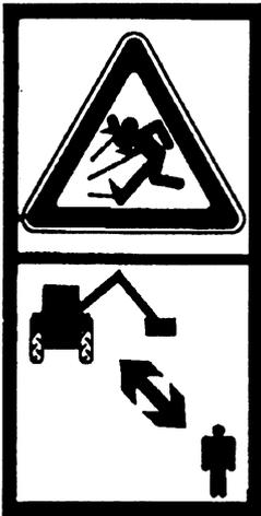
**DANGER FROM THROWN DEBRIS. KEEP ALL PERSONNEL AT A SAFE DISTANCE FROM THE MACHINE WHEN WORKING**
