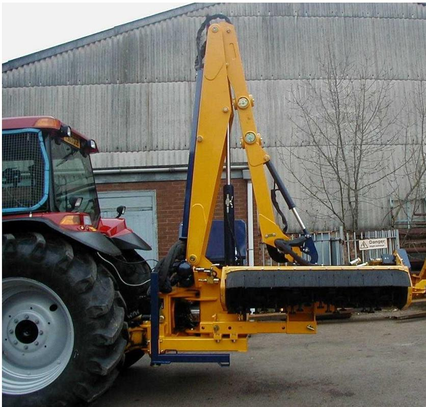
**Cutting Head Placed On Support Bracket**
