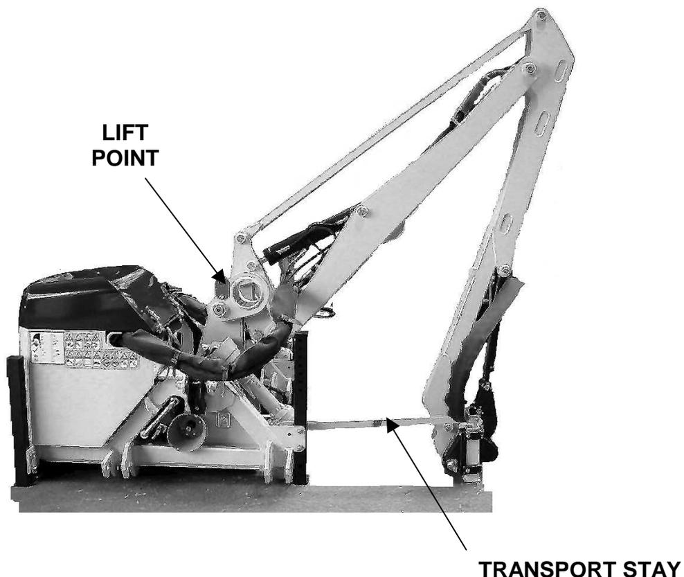
**MACHINE PREPARATION: THREE POINT LINKAGE****IMPORTANT**
