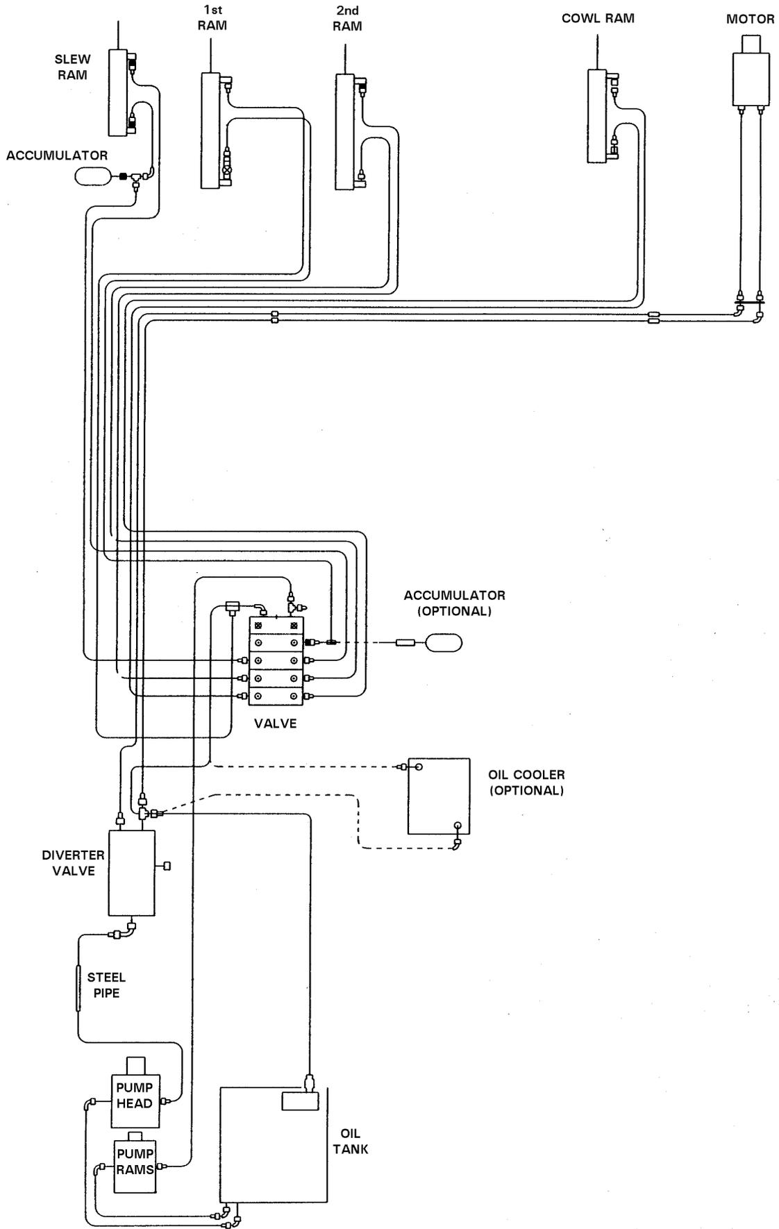
**HOSE CIRCUIT DIAGRAM (Power Slew Machines)**
