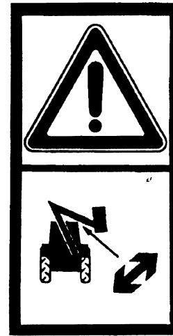
WARNING! ARMS MAY HIT CAB IF CLEARANCE IS NOT SUFFICIENT
