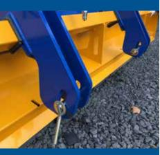
**Float function**Slotted holes for simple float function.
