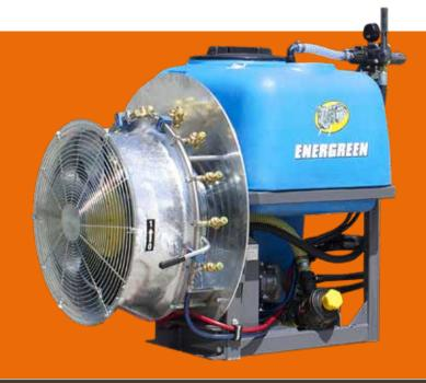
Sprayer with frame in steel and tank in polyethylene and total emptying, fan with nine galvanized blades, suitable to carry out pesticide treatments and fungicides on vineyards and fruit trees. It can be equipped with an herbicide bar (optional) with an extensible part and the possibility of using only the right or left bar through a control opens the taps. In addition, the sprayer can mount a reel (optional) with manual water gun, to work in the most inaccessible and rough areas.
