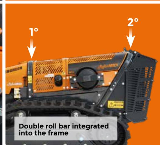
Double roll bar integrated into the frame
