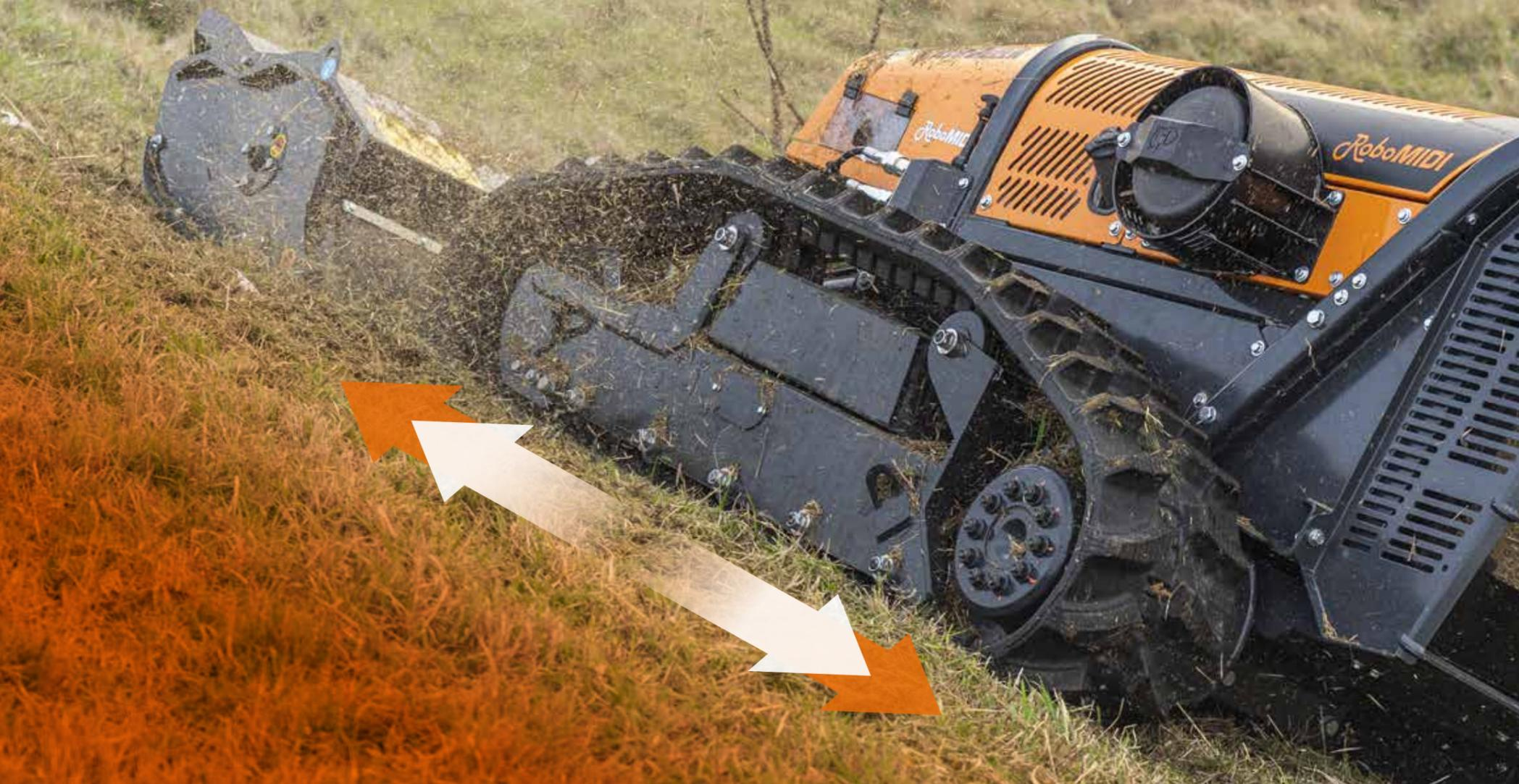
**Tracks profile with the largest contact surface and smallest specific weight on the ground**
