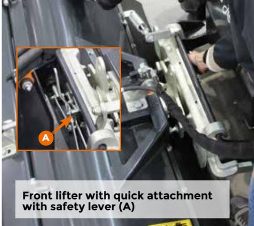
Front lifter with quick attachment with safety lever (A)
