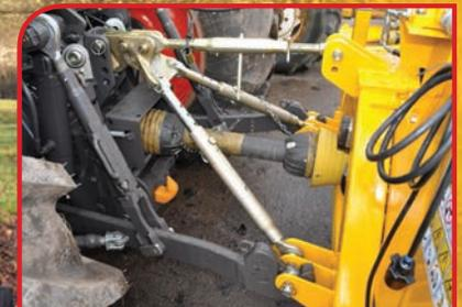
Swing system and a tubular 3 pt. linkage kit standard.
