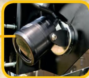
Features include right side viewing camera. Standard equipment on the RailKut. Allows operator clear view of cutter head in operation while facing forward and steering vehicle.
