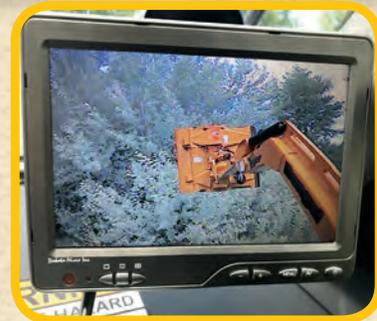
Viewing Monitor located in cab of truck.
