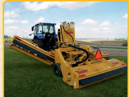
Developed to handle today's mowing challenges with quick disconnects for easy detachment and built with your transportation needs in mind. When mowers are up and locked, unit is legal width, ready to travel safely from job site to job site. Tiger Extreme Duty Flails are designed and built to meet and exceed ANSI and SAE standards.
