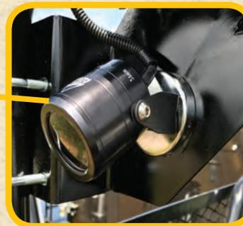
Optional camera located on the right side of the TruckKat allows the operator to view the cutting head in operation while facing forward and steering vehicle.
