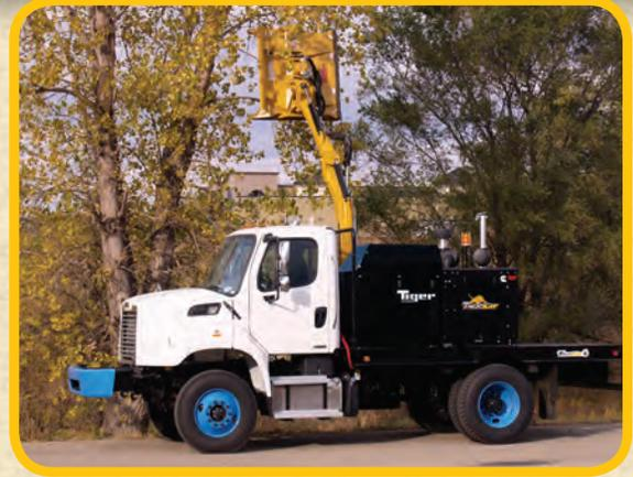
The Tiger TruckKat Boom Mower can be purchased as a turnkey unit with the Ford F550 FWD chassis, or as a truck bed mount designed for 36,000 GVW trucks with dual steering similar to the Freightliner M2 series.
