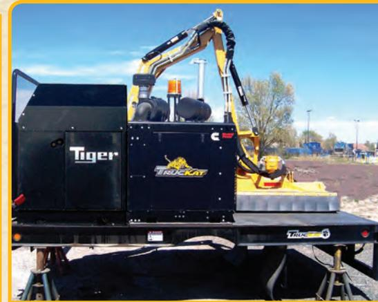
Remove the Tiger TruckKat in minutes with the use of the patented Kybato Quick Change system. The quick disconnect system allows the truck to be used for other applications throughout the year.
