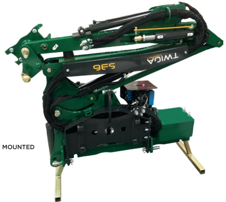
The Twiga Compact series comes as standard with the Minipilot Electric Proportional control system, giving all day comfort. Operating functions are easy to hand on the incorporated control box.
