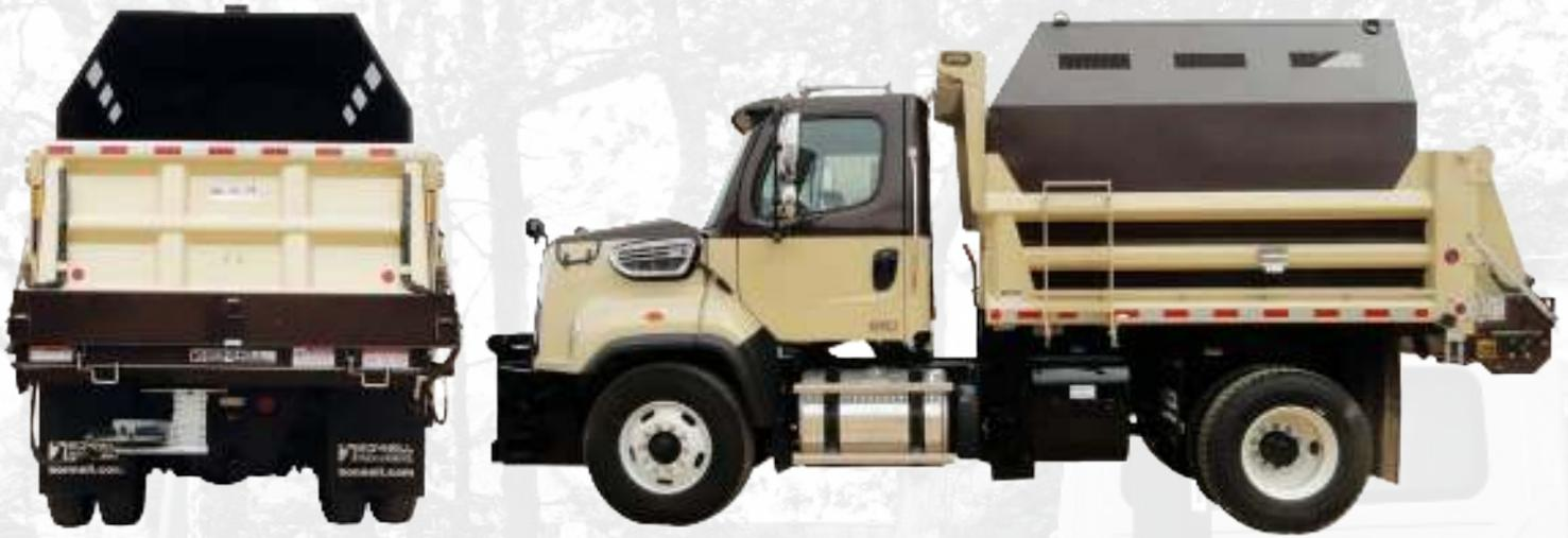
Collect and haul your mulch, brush and chips in style. Each Titan Chipper Cap is custom built for an exact fit to your existing dump body. Remove the side boards, drop in place, bolt on, and go. Designed to contain stray debris and chips and look good too. The Titan Chipper Cap is fabricated from 10-gauge carbon steel.
