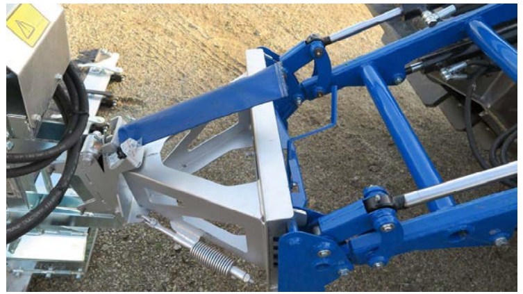
Lifting arm with parallel movement. Semi-automatic quick bracket X4 for fast tool replacement.
