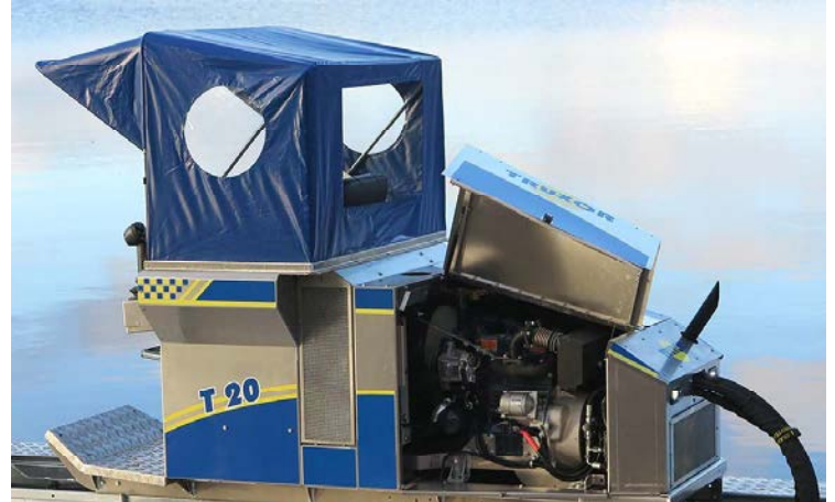
Easily accessible engine compartment facilitates service.
