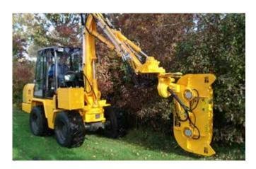
Herder develops machines based on a wide range of vehicles. This an example shows a loader as the basis. The removal of the original loading boom made the vehicle suitable for vegetation maintenance, for instance.
