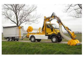
Herder developed this machine for working on road shoulders with minimal traffic measures.
