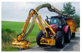
An example of a specially commissioned machine, with the boom constructed on the nose of the tractor. This makes it possible to mow in (narrow) sunken roads.
