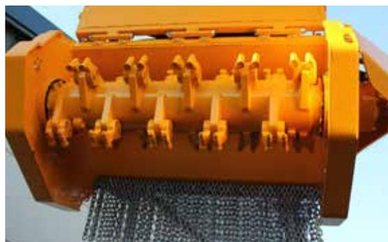
*Close-up of rotor shaft with teeth*
