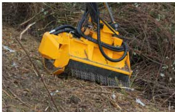
*The back of the forestry mower has a heavy chain guard for safety*
