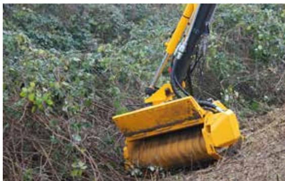
*The hydraulic folding front can be opened, as shown here, to feed tall shrubs in more easily*
