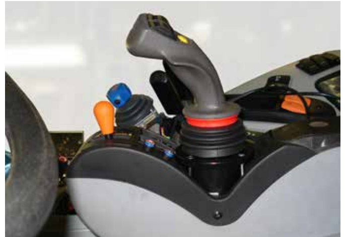
Electric joystick control is available as an option. Another option is extra float position control next to the right-hand joystick, so the control panel can be placed at the back of the cabin.
