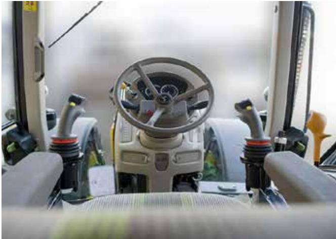
Electric joystick control is available as an option. Another option is extra float position control next to the right-hand joystick, so the control panel can be placed at the back of the cabin.
