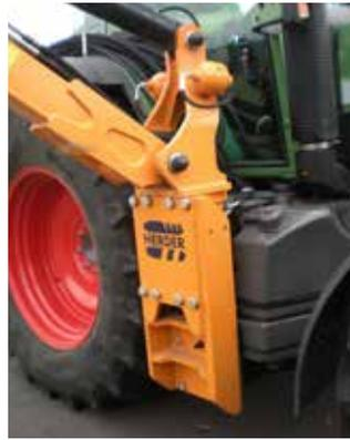
*Pivot 'rotating cylinder' for narrow mounting.*
