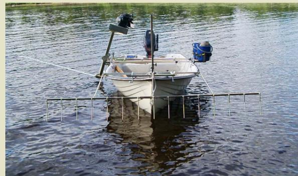
The **Dorocutter Klippo** is a machine in the middle class. All maneuvering of **Klippo** is done from the drivers seat, like deep-going and the drift of the knife. The knife can be angled for cutting in blanket of plants and cutting close to land. **Klippo** is equipped with rockreleasing and has an adjustable frame for different boatwidths.
