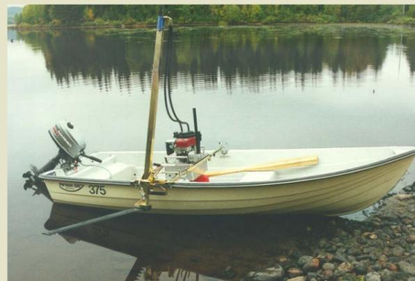
The **Dorocutter Hymo** is our deep cutting machine. Our hydraulic unit **Hyddo 200** is used as source of energy. The machine is very reliable because of the hydraulic operation. The **Dorocutter Hymo** is delivered complete with the hydraulic unit. Rock releaser is standard. The **Dorocutter Hymo** is also available with extended working depth.
