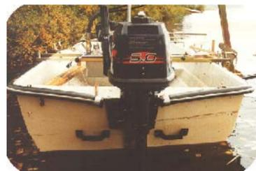
Sidemounted reedcutters pull the boat sideways. This is compensated if the boatengine is mounted a little bit to the right.
