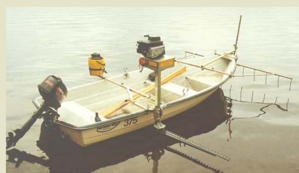
The **Dorocutter Wasse** is our smallest engine powered reedcutter. **Wasse** is the suitable reedcutter when small areas and different watersystems are maintained. The cutting deep, the drift of the knife, start and stop of the engine etc. are done from the drivers seat. The light construction makes transport and mounting easy. Rockreleaser is standard.
