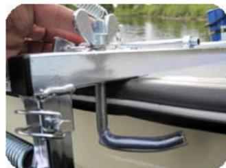
The gunwalehook squeeze the frames stuck from the underside of the gunwale. All frames are telescopic to suit different boatwidths.
